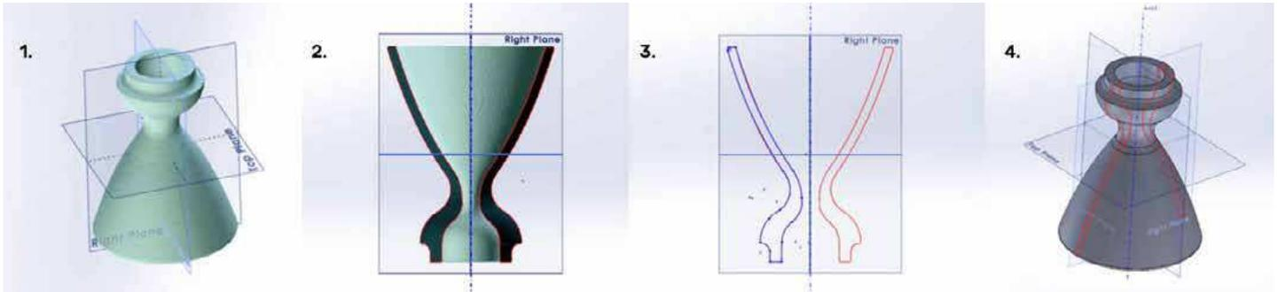
1. Create a new coordinate system. It makes it easier to reverse engineer your part in later steps.
